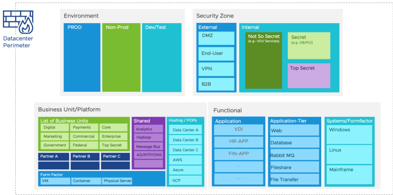
Figure 1-2: The datacenter security classification layout
