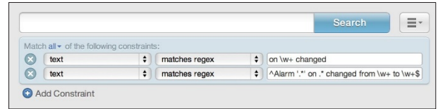
Figure 8. An example of two different ways to query for the same field. The first constraint is generic and contains only two keywords. The second constraint is specific and has five keywords. The second constraint is always preferred over the first.
