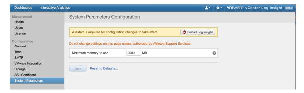
Also note that for L (large) installation, you need to upgrade your VM hardware version. By default, Log Insight uses VM hardware version 7 so that the VM can run on any ESXi 4.x and 5.x host, but it can only support up to 8 CPUs. You'll need to upgrade it to VM hardware version 8 (for ESXi 5.x) or 9 (for ESXi 5.1) in order to provision 16 CPUs. You'll have to power off the VM to do so.
