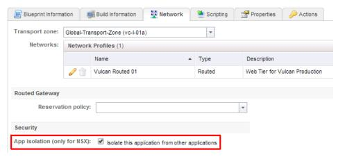
In this example I have defined a single Routed Network Profile in the Blueprint, which means that one VXLAN Logical Switch will be created dynamically for each Deployment instance deployed from this blueprint connected to an NSX Distributed Logical Router.
