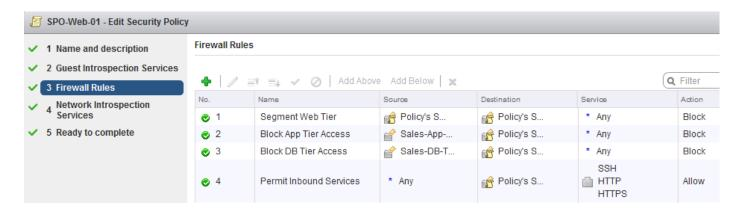
Firewall Rule 1 blocks any communication between Web VMs, Rule 2 blocks access from the Sales-App-Tier-01 VMs to Web VMs, Rule 3 blocks Sales-DB-Tier-01 Access and Rule 4 Permits selective Inbound Services from External Networks (any). This policy has a weight of 4300.
