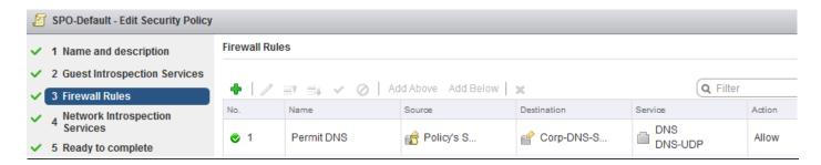
Finally, when **App Isolation** is enabled on a vRealize Automation Blueprint, the following Security Policy is automatically created the first time a Multi-Machine Service is deployed, so no configuration is required:
