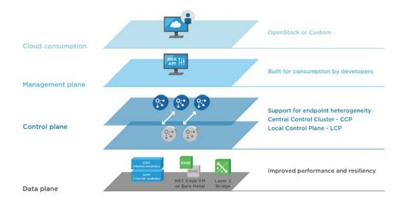
As seen in the graphic, the NSX-T architecture is made up of the management plane, control plane and data plane. This separation allows the architecture to grow and scale without impacting workloads. We'll describe each layer and its components below.
