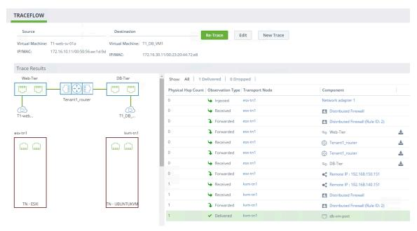
An example of Traceflow in action is shown in the figure where a trace is being run between 2 VMs running on ESX and KVM hypervisors which are attached to Web-Tier and DB-Tier logical switches.
