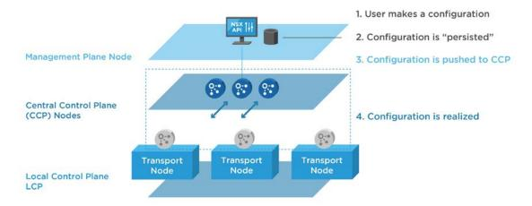
The NSX-T control plane encompasses a clustered control-plane (CCP) running on controller nodes and a localized control plane (LCP) on compute endpoints.
