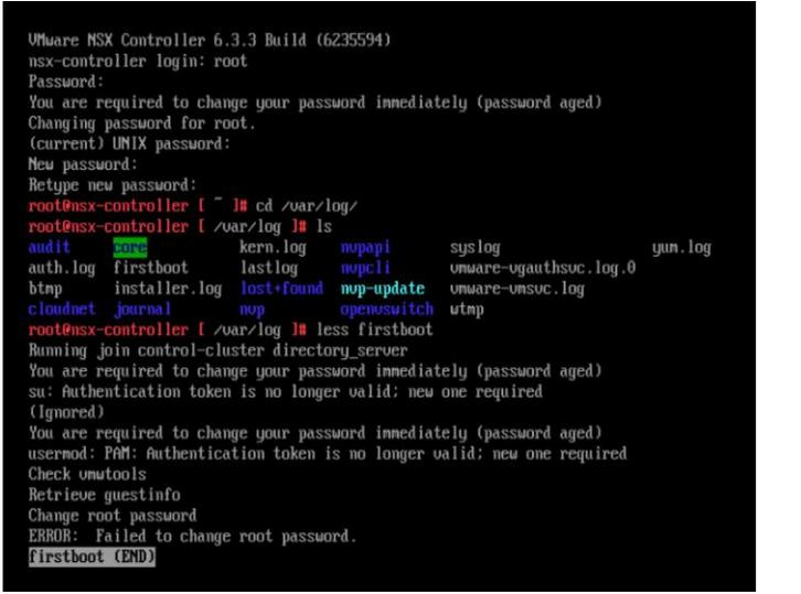
12. When I ran the “chage –l root” command in the console, found that “root” password is set to expire in 90 days. This may be issue that causing the controller VM is not assigned with IP Address.
