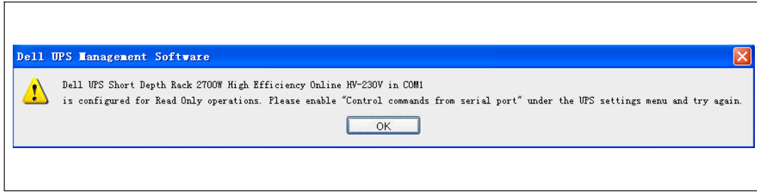
Figure 82. UPS is Set to Read-Only Message
