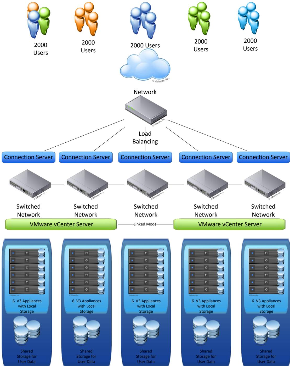
**Figure 1. High-level Proposed Architecture for V3 Systems' Full 10,000 Virtual Desktop Configuration**
