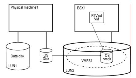
Figure 4: Use P2V to build the new VM and load the OS
