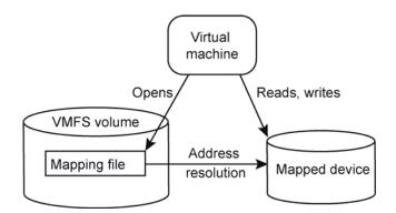
Figure 3: The RDM file in a VMFS volume provides a symbolic link to the raw mapped device.
