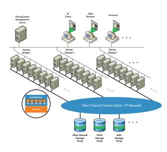
As Figure 1-2 shows, a typical VMware Infrastructure data center consists of basic physical building blocks such as x86 computing servers, storage networks and arrays, IP networks, a management server and desktop clients.
