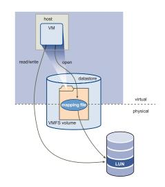
An RDM can be thought of as a symbolic link from a VMFS volume to a raw LUN (see Figure 1-11). The mapping makes LUNs appear as files in a VMFS volume. The mapping file—not the raw LUN—is referenced in the virtual machine configuration.
