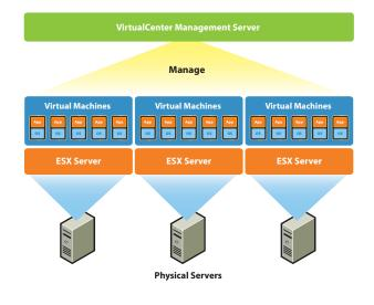
Computing servers will continue to function even in unlikely event that VirtualCenter Management Server became unreachable (e.g., the network is severed). Computing servers can be managed separately and will continue to run their assigned virtual machines based on the resource assignments that were last set. Once the VirtualCenter Management Server becomes available, it can manage the data center as a whole again.
