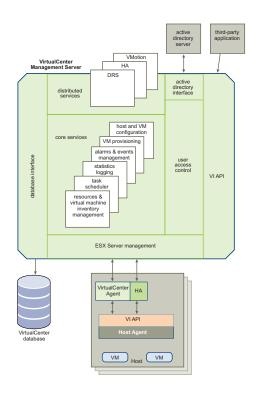
Figure 1-14 shows the key functional components of the VirtualCenter Management Server. They include User Access Control, Core Services, Distributed Services, and interfaces to external resources..
