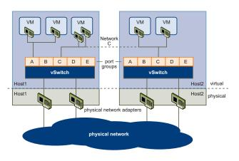
Figure 1-9 shows the relationship between the networks inside and outside the virtual environment. The virtual environment provides similar networking elements as the physical world. They are virtual network interface cards (vNIC), virtual switchs (vSwitch) and Port Groups.
