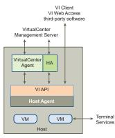
ESX Server communicates with other resources through its Host Agent using the VMware Infrastructure API (VI API). Using the VMware Infrastructure SDK, both VMware and third-party software can collect information from and manage ESX Server through the VI API.
