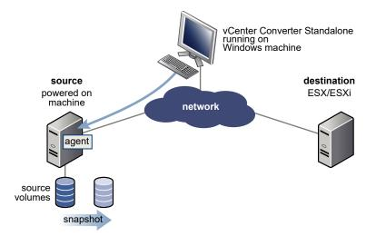
2 Converter Standalone prepares the virtual machine on the destination machine.
