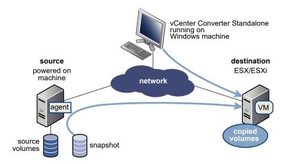
If the proxy mode feature is off, the data traffic passes from the source machine directly to the destination server.
