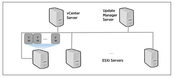
Figure 1. VUM on Windows for vCenter Server for Windows platform
