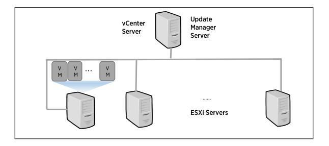
Figure 2. VUM integrated as a service in vCenter Server 6.5 for Linux platform
