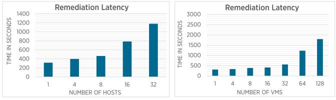
Figure 4. Concurrent remediate latency with different number of hosts and virtual machines (VMs)
