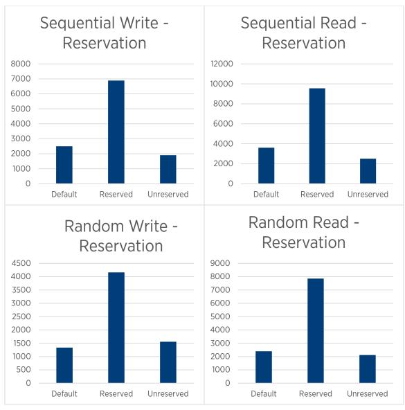
Figure 4. Performance impact of setting Limit in SIOC
