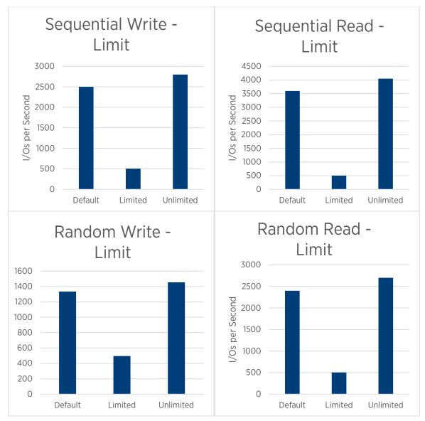
Figure 3. Performance impact of setting Limit in SIOC
