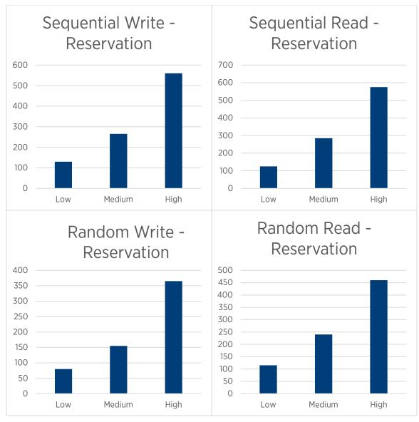
Figure 5. I/O performance using policies
