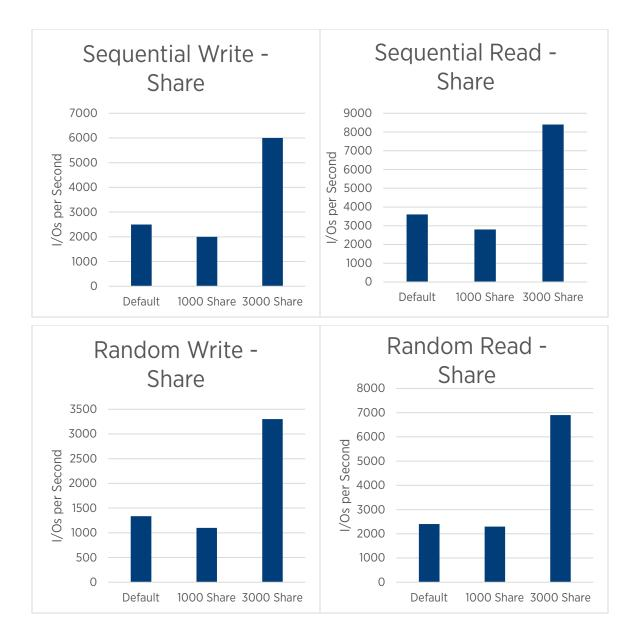
Figure 2. Performance impact of setting share in SIOC (y-axis shows IOPS)
