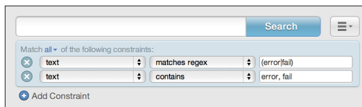
Figure 7. An example of two different ways to construct the same query. The first constraint is a regular expression while the second is a keyword, comma separated, logical OR match. The second constraint is always preferred over the first.
