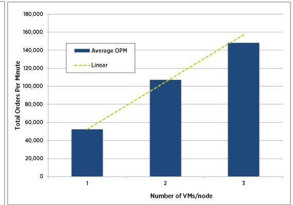
Figure 5. Scaling wrt. number of VMs/node – 4 node VSAN cluster
